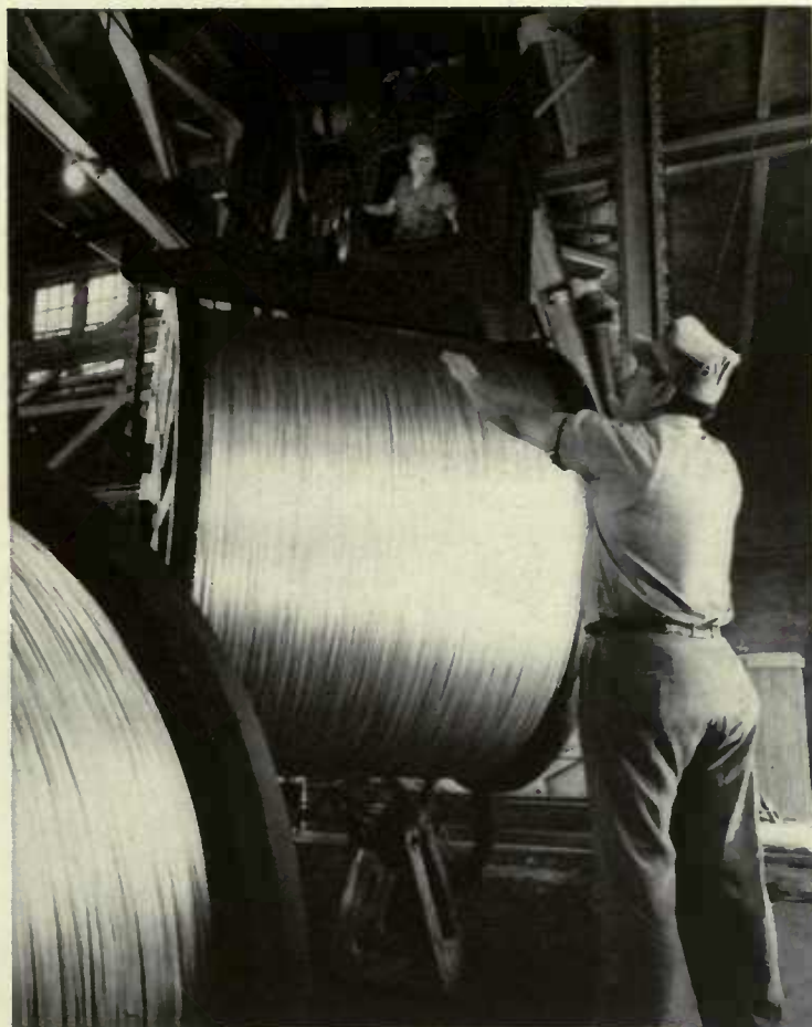
Coils of exceedingly strong steel wire for suspension bridge cables are produced to exacting requirements.
